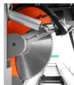
Blade handling by screw and brushless motor. Ball bearing system for precision and fluidity of movement
