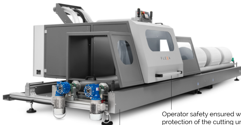
Frame in aluminium profile, tubular and powder-coated steel sheets
